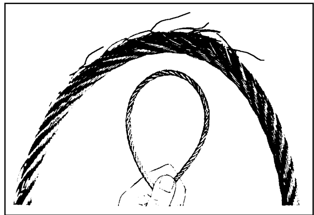
FIGURE 7-16. Cable inspection technique.
